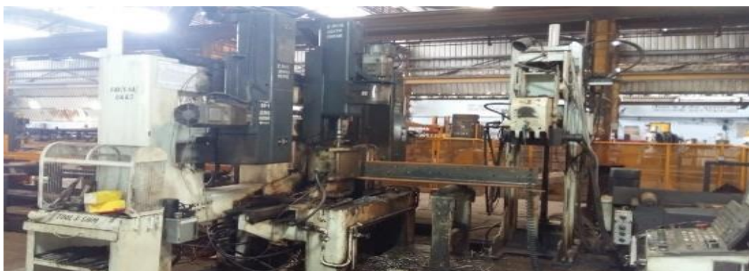
Fig 1: FICEP DB – 363 CNC Drilling Machine
